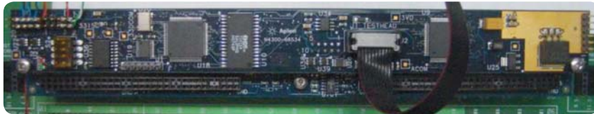
Figure 6. Flex cable connection on CET card
